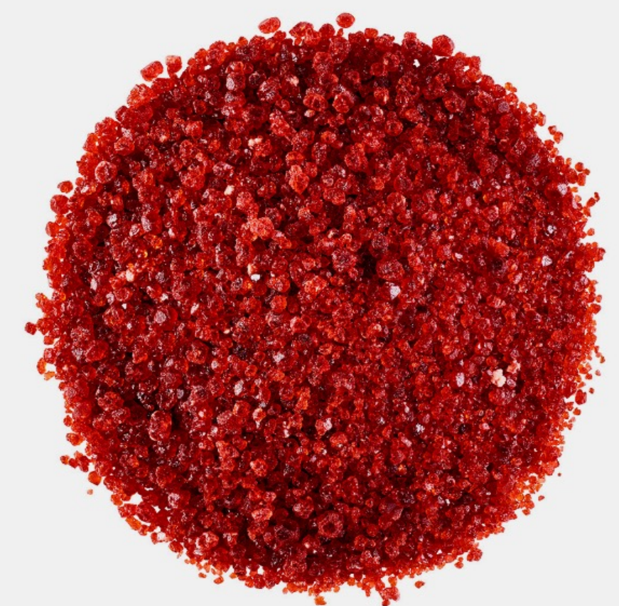
Cobalt sulfate crystals from nodules
