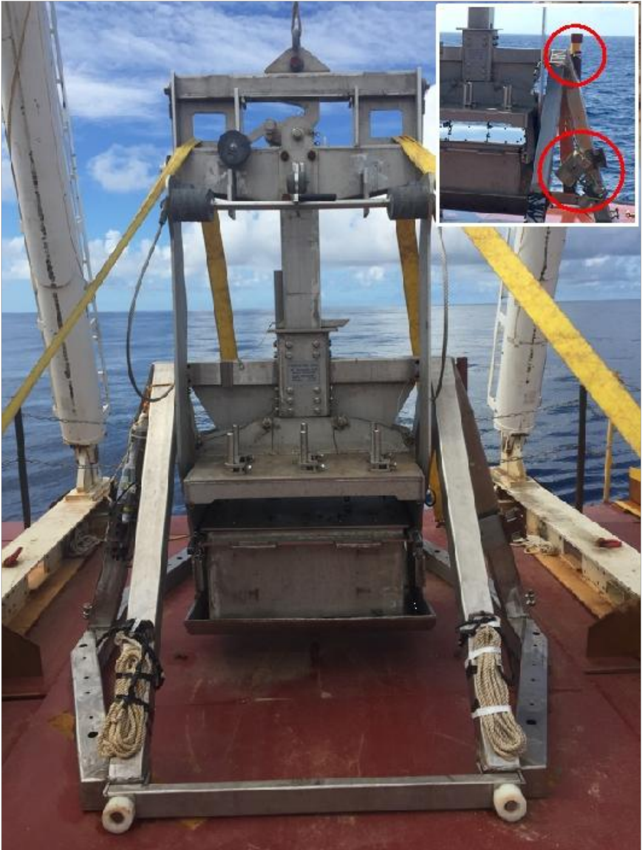
Figure 7.3 KC Denmark 0.75 m 2 box corer
