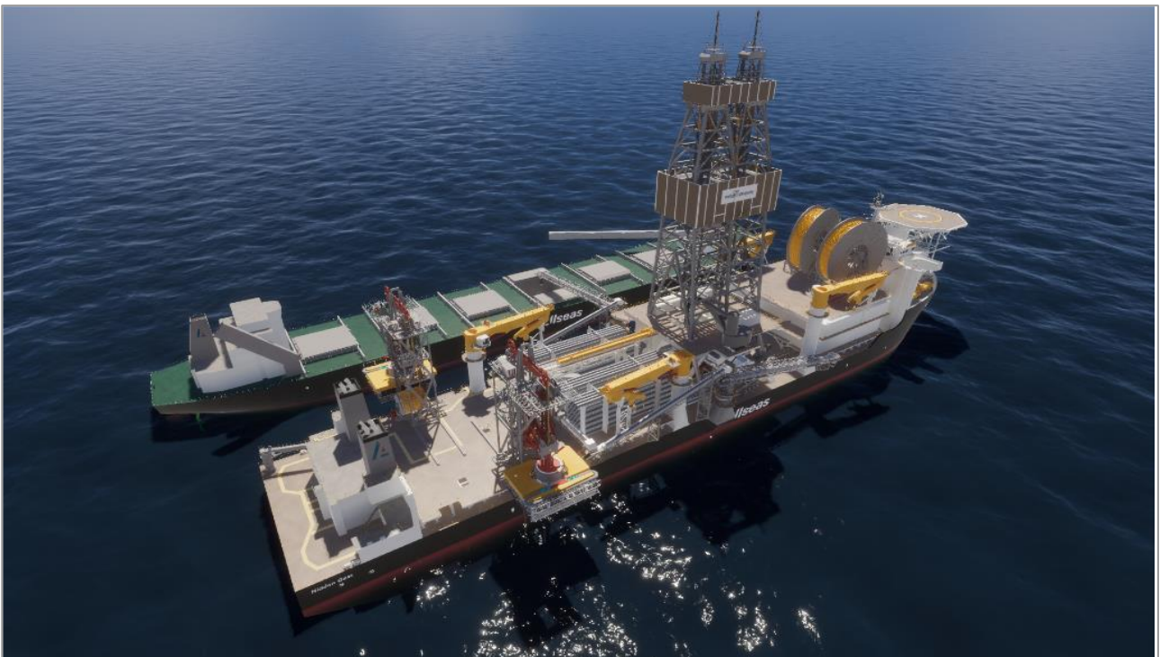
Figure 13.3 Illustration of the First-Generation Production System during nodule offloading operations.
