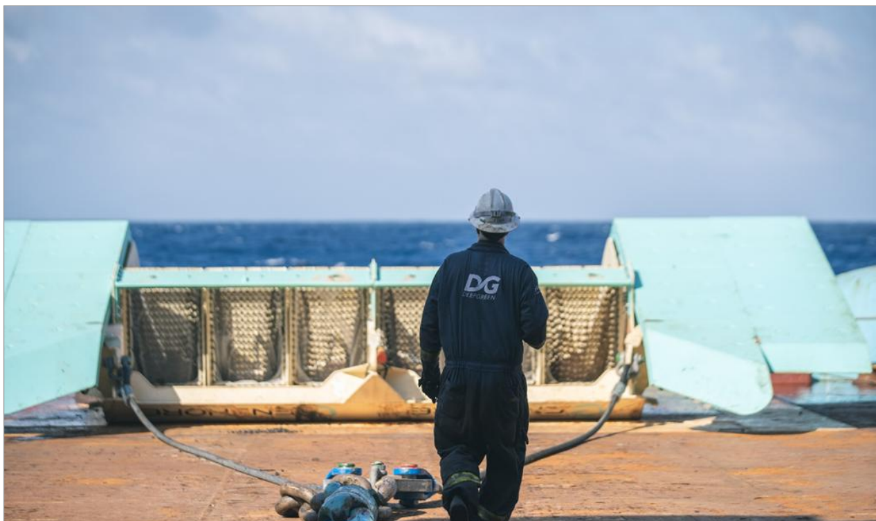
Figure 10.1 Bulk sampling dredge used to collect the bulk sample for metallurgical pilot tests
